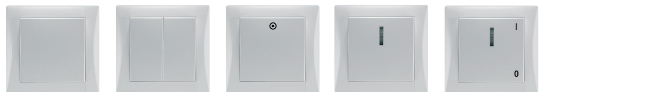
single switch, IP 44 (arrangement 1, 2, 6, 7, 1/0) double switch IP 44 (arrangement 5, 6+6, 1/0+1/0, 1+1/0) switch with target symbol, IP 44 (arrangement 1, 1/0) switch, IP 44 with backlighting (arrangement 1S, 1/0S) IP 44 switch with backlighting and I-0 symbol (arrangement 1S, 2S)
